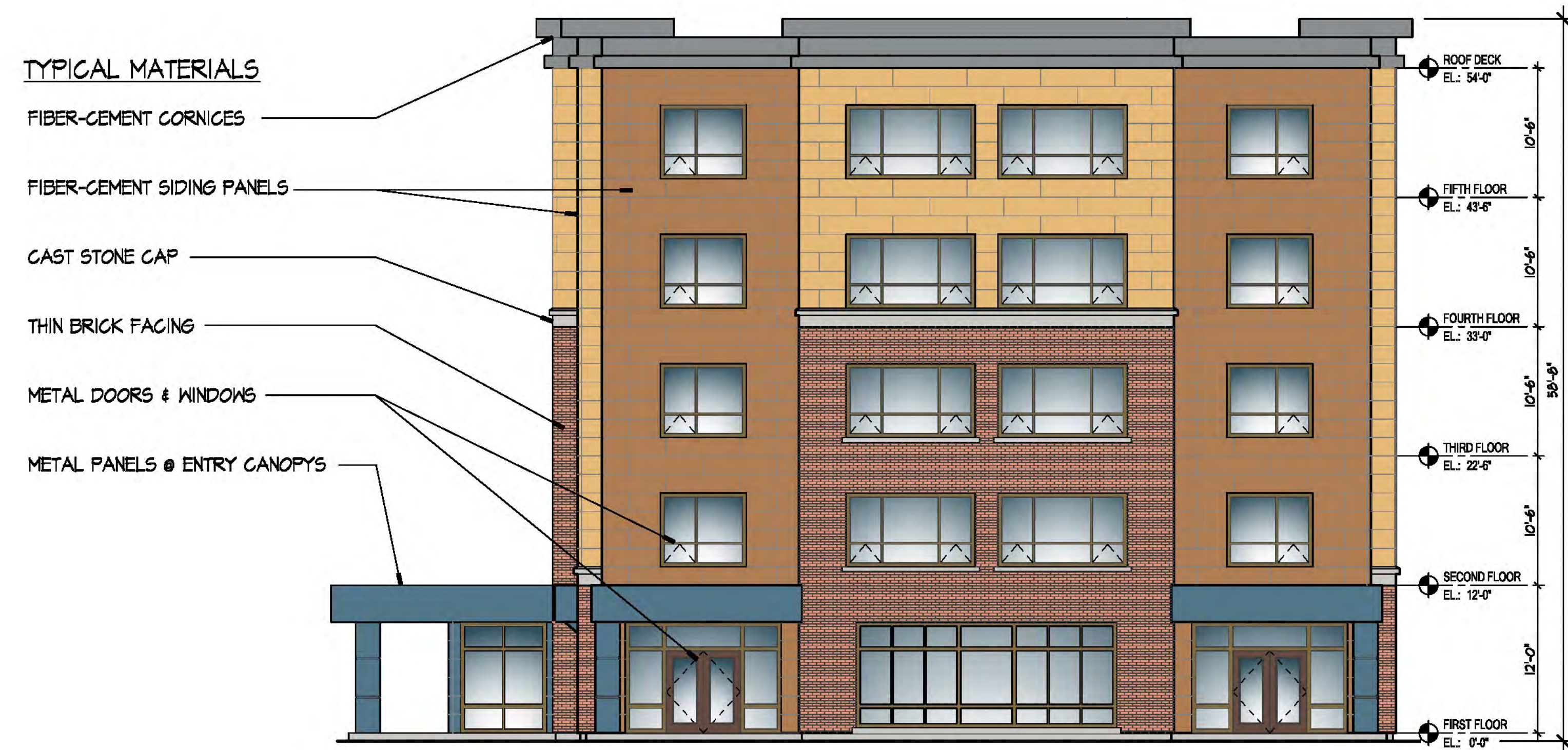
2 BUILDING A WEST ELEVATION SCALE:
